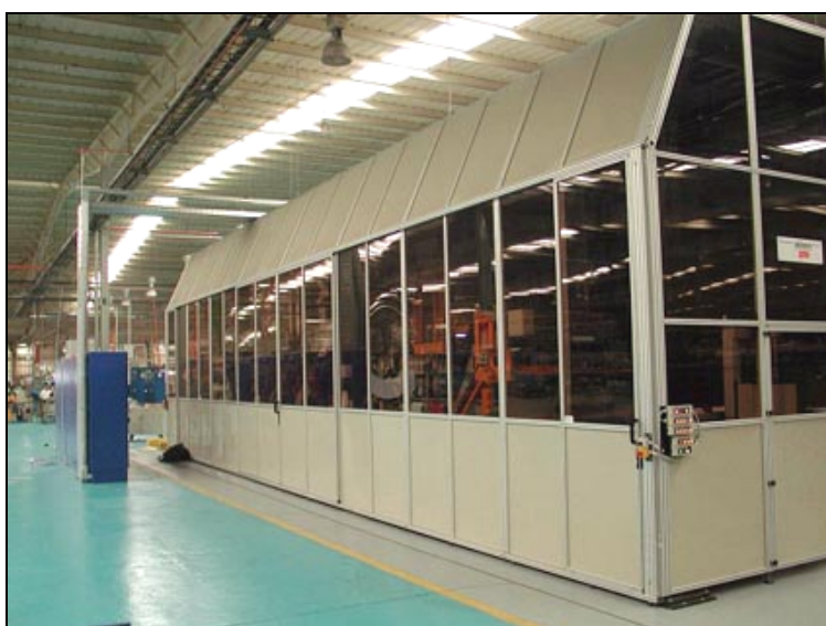
Figure 4.2 Encapsulated integrated chromium plating line [140, Atotech, 2003]
